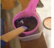
The resin Dave uses is Isopon Fastglas, coloured with powdered poster paint (which is difficult to get hold of these days). He also uses glitter or crushed tapioca to give it a bit more character.
