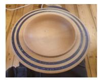
The reason that this bowl needs to be finished is that resin can have bubbles in, and so when you take the resin down on the lathe, it can expose holes, which will need filling.
